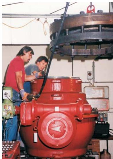
Final expection (pressure testing) of a KLINGER Ballostar KHSVI ball valve acc. to DIN 3230
