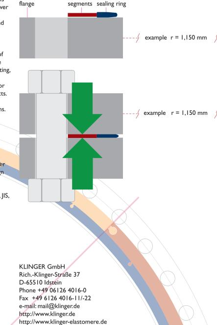
The principle of the off load gasket design
